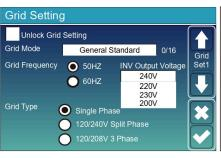
**Unlock Grid Setting:** before changing the grid parameters, please enable this with password of 7777. Then it is allowed to change the grid parameters.
